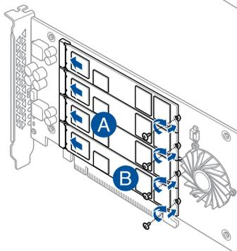
4. Peel the plastic films off the thermal pads, secure the cover to the ASUS HYPER M.2 X16 CARD V2 with the cover screws that you removed earlier, then install the ASUS HYPER M.2 X16 CARD V2 into a PCI Express 3.0 slot.
