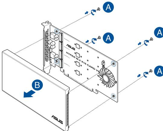
2. Secure the stand screws onto the ASUS HYPER M.2 X16 CARD V2.
