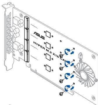
3. Insert the M.2 storage devices into the PCIe M.2 storage device connectors, then secure the M.2 storage devices with the bundled screws.
