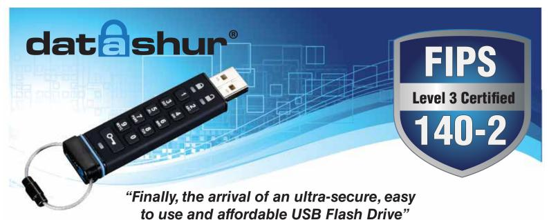
The iStorage datashur is the world's most secure, easy to use and affordable USB flash drive, employing PIN code access with military grade AES 256-bit hardware encryption. The datashur incorporates a rechargeable battery allowing the user to enter a 7-15 digit PIN onto the on-board keypad before connecting the drive to the USB port.
